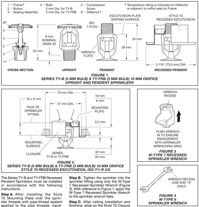
tighten the sprinkler into the sprinkler fitting.
