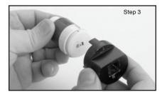
**Step 3.** Ensure that the TYCO W-Type 25 Installation Wrench is fully engaged onto the sprinkler. Fully insert all three Wrench Prongs into the slots on the sprinkler body.
