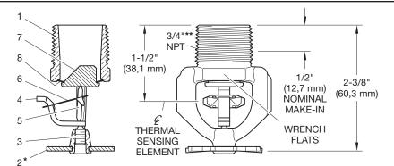
FIGURE 1 MODEL ESFR-17 PENDENT SPRINKLER, 16.8K, 165°F (74°C) EARLY SUPPRESSION, FAST RESPONSE
