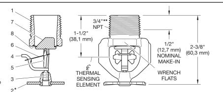
FIGURE 2 MODEL ESFR-17 PENDENT SPRINKLER, 16.8K, 212°F (100°C) EARLY SUPPRESSION, FAST RESPONSE
