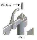
4) Squeeze reset tool handles until Operator Pin resets (clicks into place)
