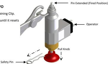
3) Align the forked end of the anvil handle around the grooved end of the Operator tip
