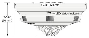
Figure 6: 4098-9734 High Temperature Heat Sensor with Base
