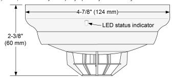
Figure 5: 4098-9733 Heat Sensor with Base
