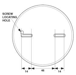
Fig. 1 Fixing Dimensions for Detector Base
